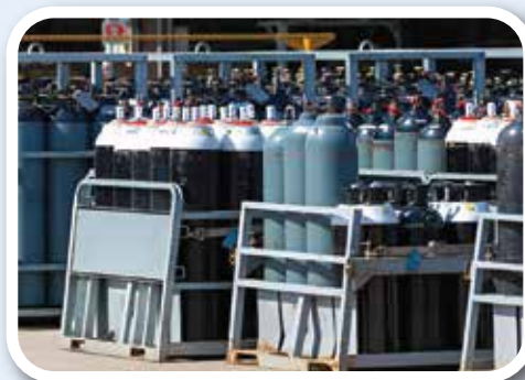
Breathing Air Cascade Racks
